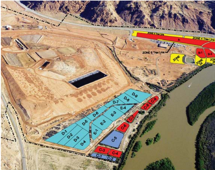
An aerial view of the uranium mill tailings pile in Moab with the Colorado River seen on the right. Red areas are previously established plots, and blue areas are new plots established in 2009 and 2010.
